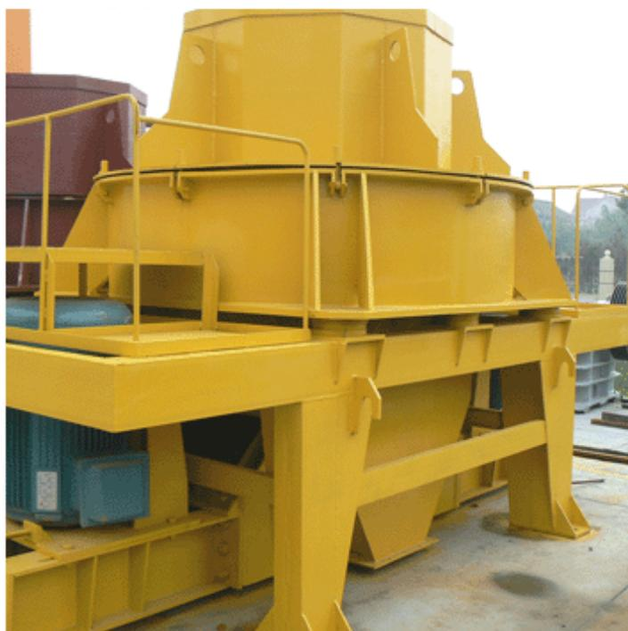
Therefore some materials will be impacted, crusher, milled twice or more times in the whirlpool cavity, then crushed materials will be excluded through the bottom discharging hole. This can form a closed circulation through the circular classifier system; in general, materials can be crushed into 20 mesh through three circulations. Airflow self-circulation in the whirlpool cavity can eliminate dust pollution well.
